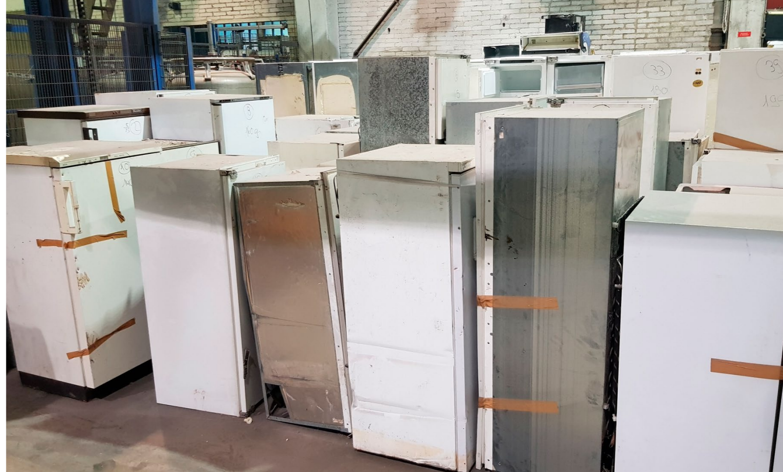
Photo 1: Temperature exchange equipment, ready for processing.
