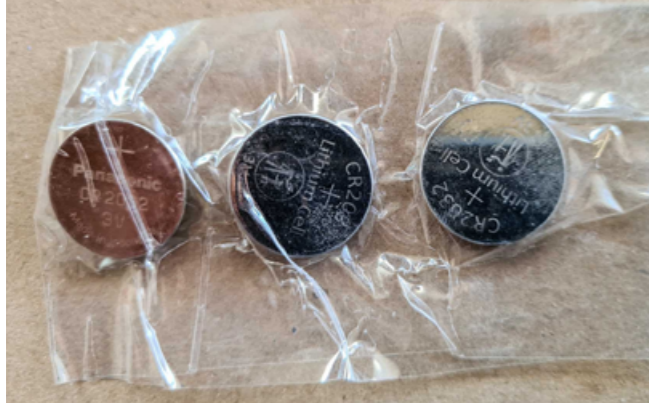
Masked off lithium button cells prevent short circuits in larger quantities (photo: soRec)
