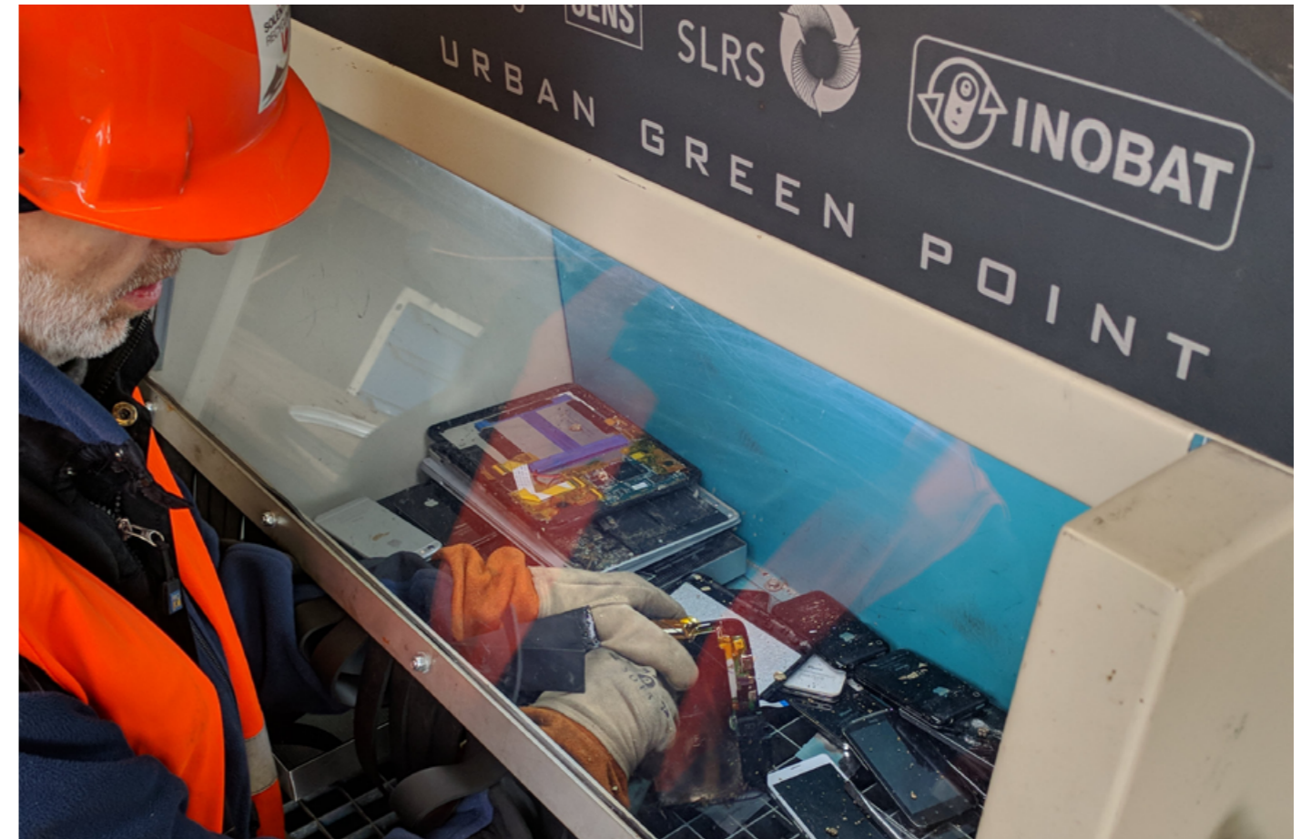
Correct handling of lithium batteries during disassembly. (Photo: Solenthaler Recycling)
