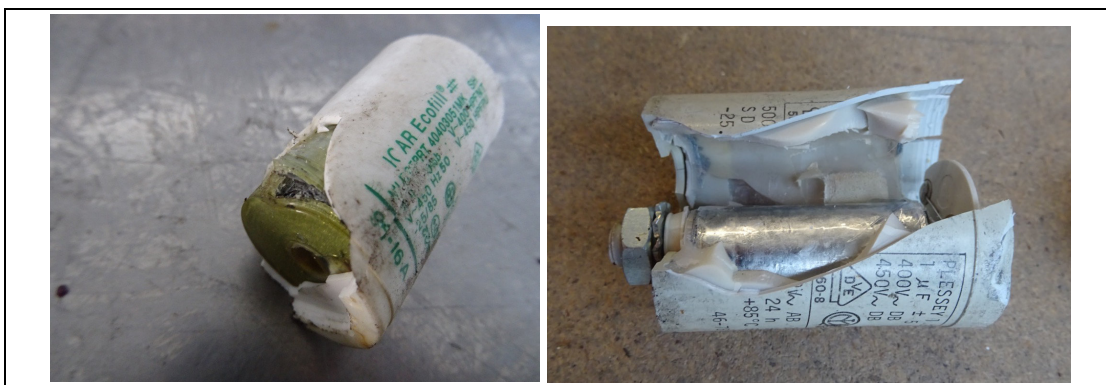
Figure 18: Opened plastic capacitors without liquid substances
