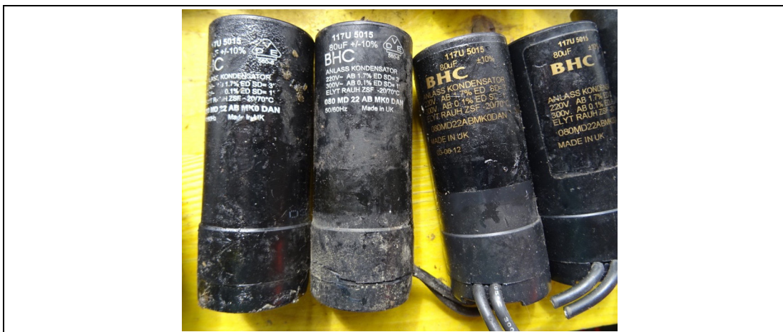
Figure 19: Motor start capacitors in black plastic housings
