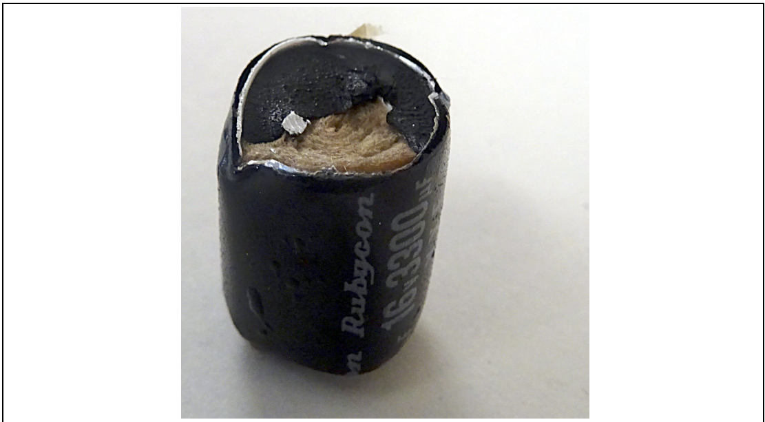
Figure 13: Aluminium e-cap, cover removed; view of bitumen seal and coil
